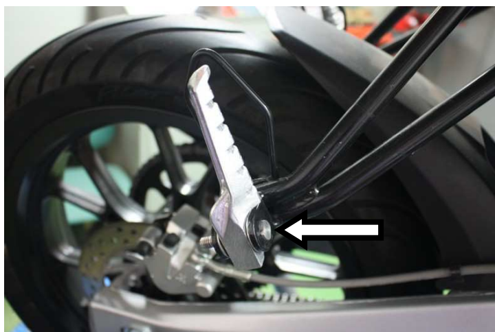
Inserire il perno fornito Fit the pin given in the fitting kit as shown above
