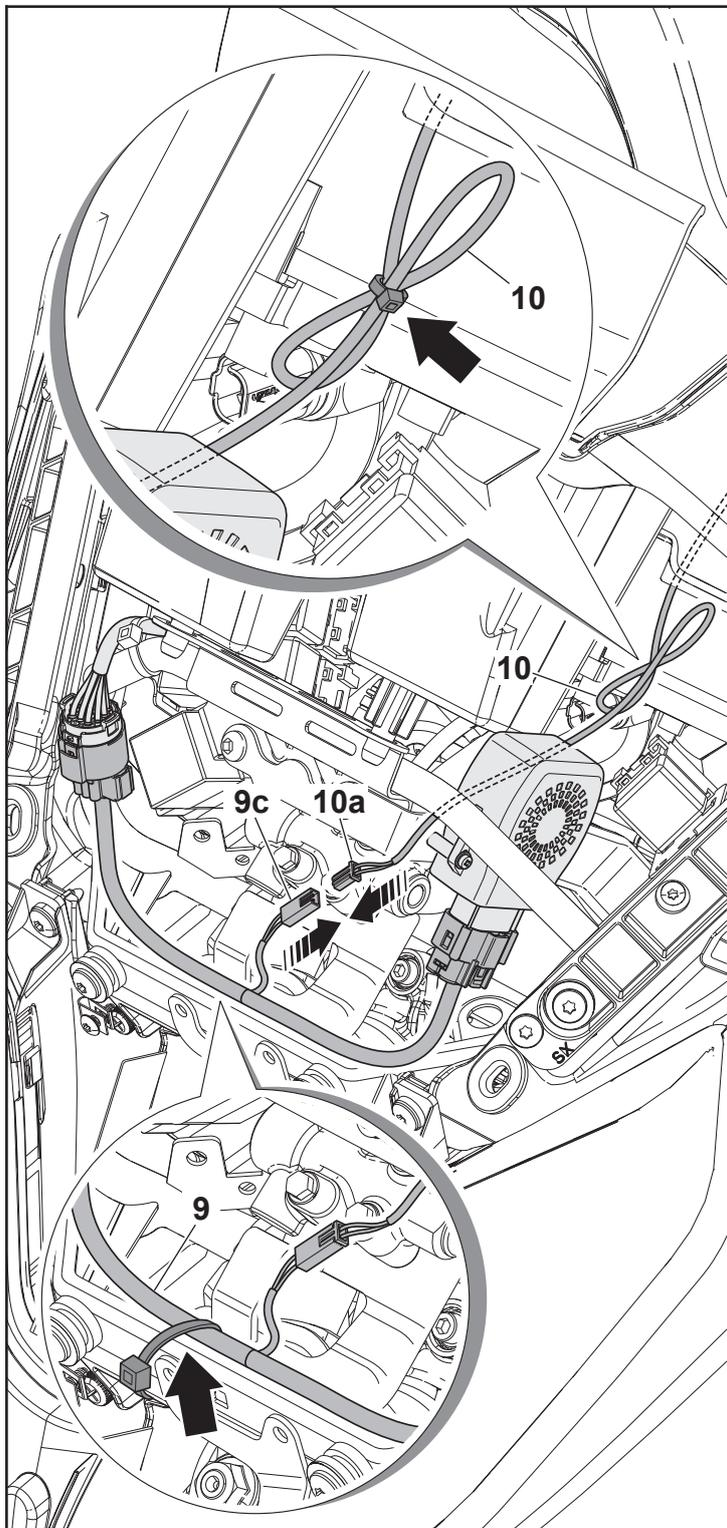
**GB** Connect the connector **10a** of the antitheft LED cable **10** to the connector **9c** of the clamp **9** of the kit and put the excess cable together with a clamp, as indicated in the figure.
