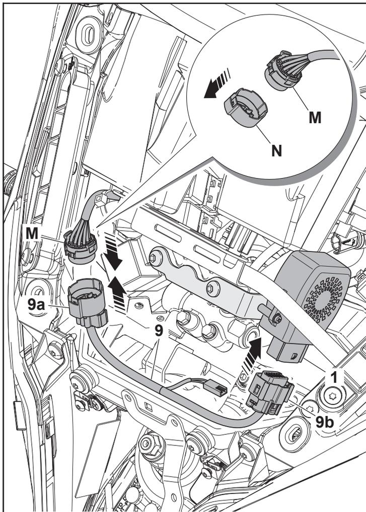
**GB** Remove the cap **N** of the connector **M** of the vehicle and store it carefully, then connect the clamp **9** of the kit to the vehicle as indicated in the figure: connect the connector **9a** to the connector **M** of the vehicle and the connector **9b** to the anti-theft control unit **1**.
