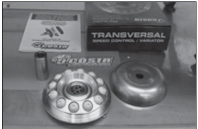
Check that the kit is complete, with all the gliding rollers present before installing the variator. If there is a slider in the kit, it must replace the original one. If there isn't, you must use the original one (check if it is really the original one not third-party one). Check if the supplied slider with the kit has the same measurements as the original one.
