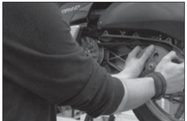
When the cover is off, you must reduce the rear pulley pressure in order to reduce the belt tension
