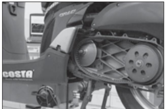
Remove the fixed pulley.
