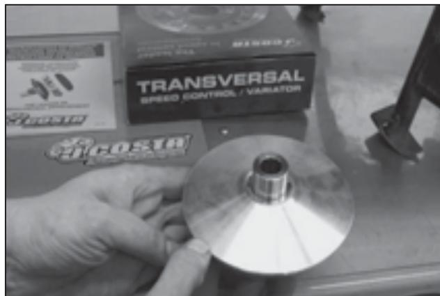
Install the bell; put the slider through the bushing as shown in the picture.
