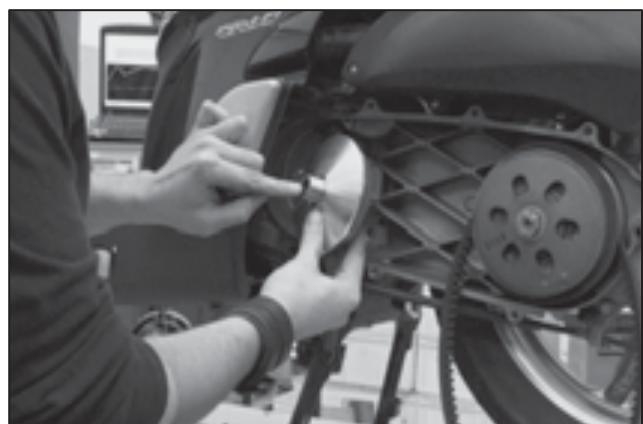
Fit the variator on the crankshaft. Install any washers to their original location (if applicable). Always in the same position as it were. J.COSTA recommends to change the original belt for the J.Costa belt (reinforced kevlar belt) in the moment of installing the variator.
