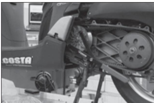
Before tightening the nut, secure the fixed pulley with the special tool.
