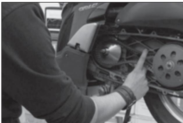
Fit the fixed pulley, washer and nut in same position as the original variator.
