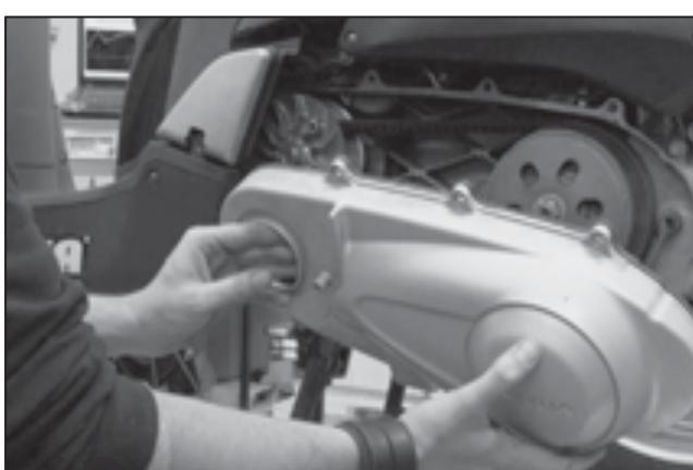
Install the cover that protects the automatic transmission system. The variator is ready to use.
