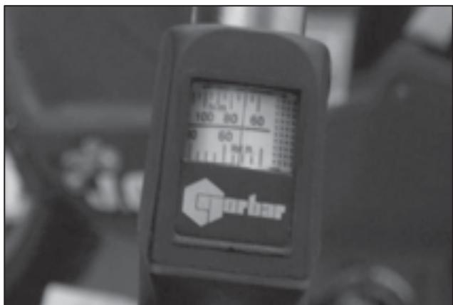
Adjust the torque wrench at the right torque before tightening the nut. You have the entire torque setting list in the manufacturer's instructions or service manual.
