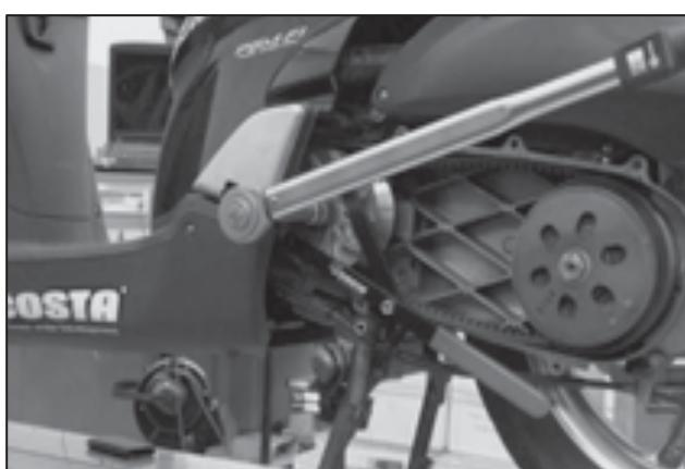
Tighten the nut with the **torque wrench**, **while holding the fixed pulley** with key tool.
